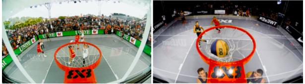
Remote controlled (or fixed) looking through or over the backboard, and able to move with the action. Camera should be mounted to feature the branded rim stickers in vision and it will be equipped with a wide angle lens.
